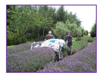
Designed to make harvesting much easier and less labor intensive our harvester is a very efficient machine suitable for small to medium size growers. Its motorized power head cuts the crop at a preset height and blows the cuttings into a collection bag.
